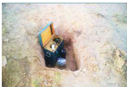
3-rasm. Guralp 6TD seysmometri yordamida shovqin darajasini o'rganish jarayoni
