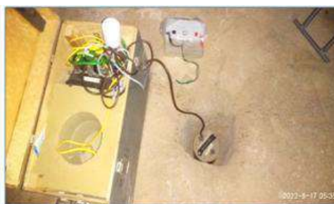
3-rasm. Guralp 6TD seysmometri yordamida shovqin darajasini o'rganish jarayoni
